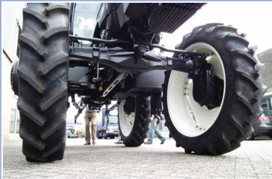
Left: A worm's eye view of the four-wheel drive County Hi-Crop conversion based on a New Holland T6030 Elite tractor showing the front axle layout.
